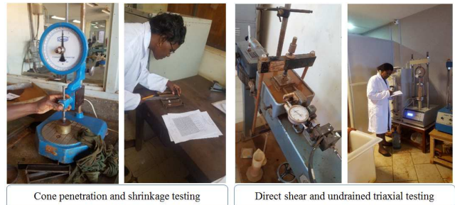
Figure 4. Plasticity, Shrinkage, Direct Shear and Undrained Triaxial Testing.
