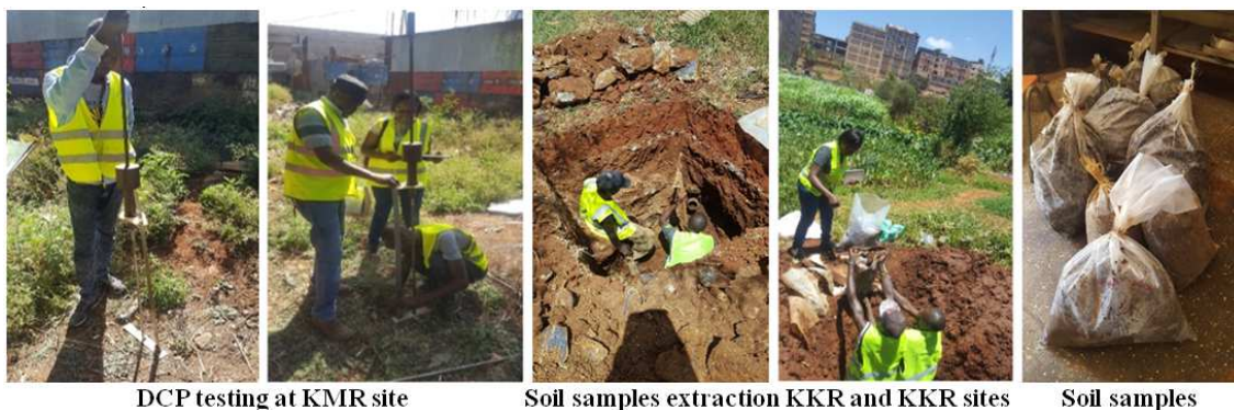
Figure 2. DCP testing and Extraction of soil samples at various sites.
