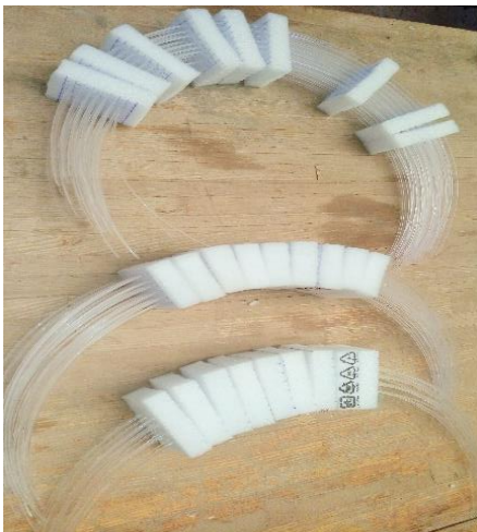
(a) Fixation of POF in low-density polyethylene (LDPE) sheets
