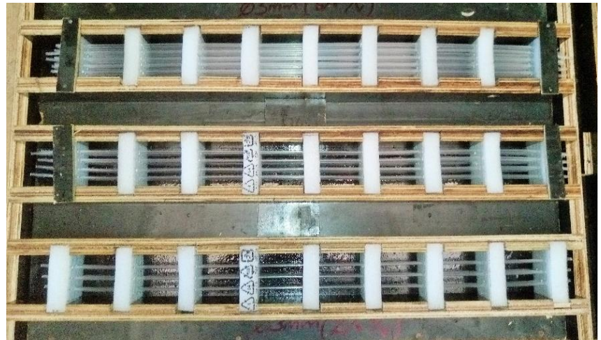
(b) Preparation of cubic mould after fixing POF
