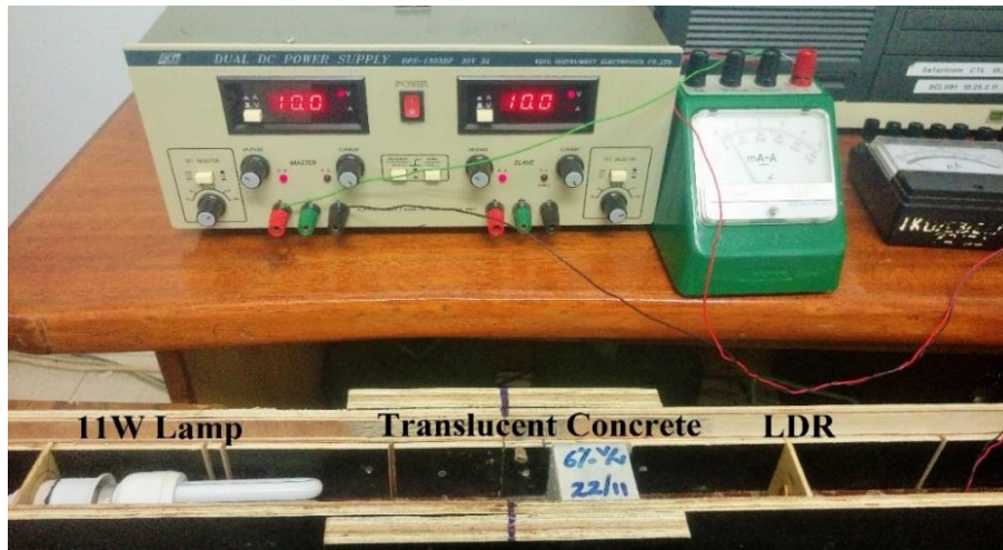
Figure 3: Experimental setup and arrangement of light transmittance test
